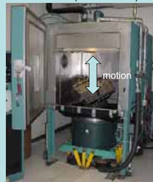
Figure 25-15A "Tilt" (not Multi-Axis) Fixture
