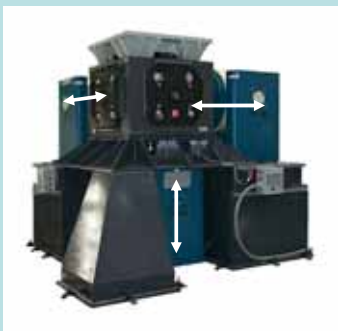
Figure 18 Three-shaker Navy 3DoF realization
