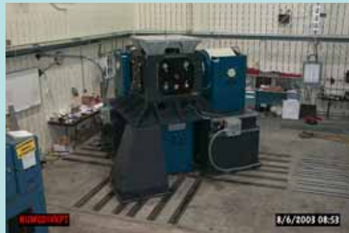
Figure 17 Three-shaker 3DoF realization
