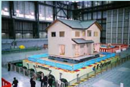
Figure 5 Seismic Investigation of Residence
