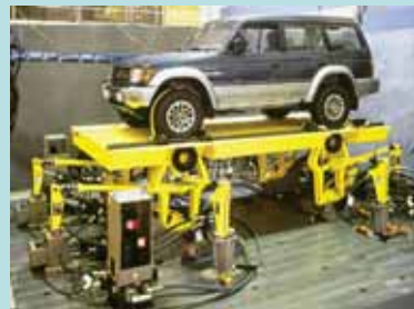
Figure 8 Platform Simulates Rail or other Transport
