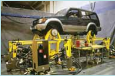
Figure 9 Road Simulation on Automobile
