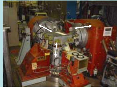
Figure 15 Pioneer Three-shaker 3DoF realization
