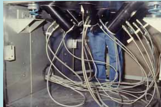
Figure 25-37 Pneumatic RS Units Excite Platform
