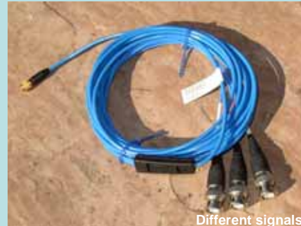
Figure 7-23B Three accelerometers → three signals
