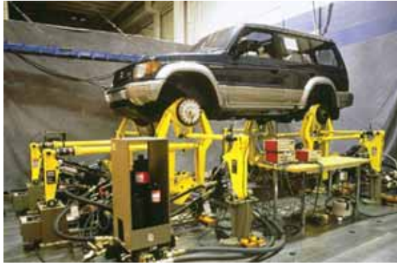
Figure 2 - Multiple servohydraulic shakers excite an automobile, simulating a variety of road and off-road inputs during various driving maneuvers. courtesy MTS
