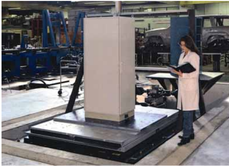
Figure 5 - A servohydraulic shaker conducts a horizontal NEBS (Network Equipment Building Systems) single axis seismic shake test. Later the cabinet (telecom equipment) will be rotated 90o. Still later it will be vibrated vertically by another shaker. courtesy Dayton T. Brown
