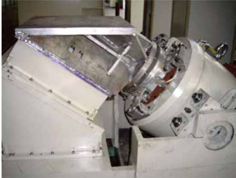
Figure 7 - Contrivance for tilting an ED shaker, thus allowing the upright DUT to move along a tilted single axis.
