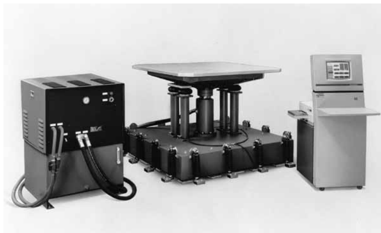
Figure 4 - A servohydraulic shaker, center, drives a platform to which DUTs will be attached. Note the reaction mass against which the shaker pushes. At left is an electric motor-driven pump and oil reservoir, while at right we see digital shaker controls. courtesy Lansmont
