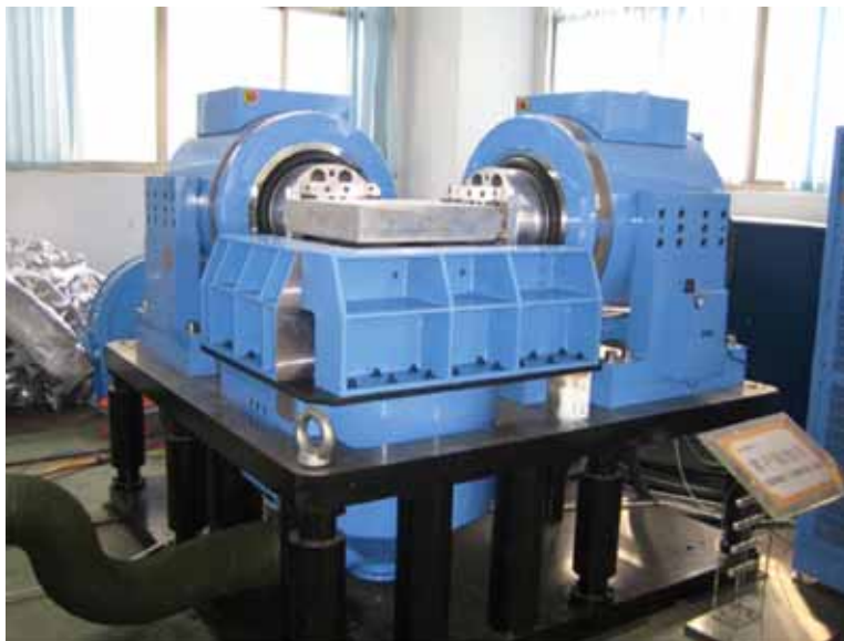
Figure 14 - Simultaneous three axis shaking is possible with this shaker system. courtesy Suzhu Dongling
