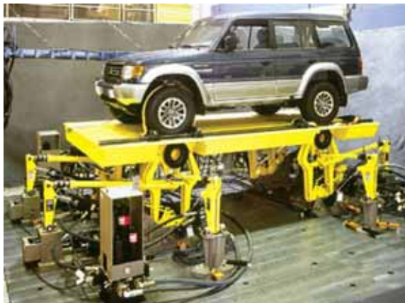
Figure 3 - Multiple servohydraulic shakers drive a platform that simulates railcar vibrations during shipment from factory to dealerships. courtesy MTS
