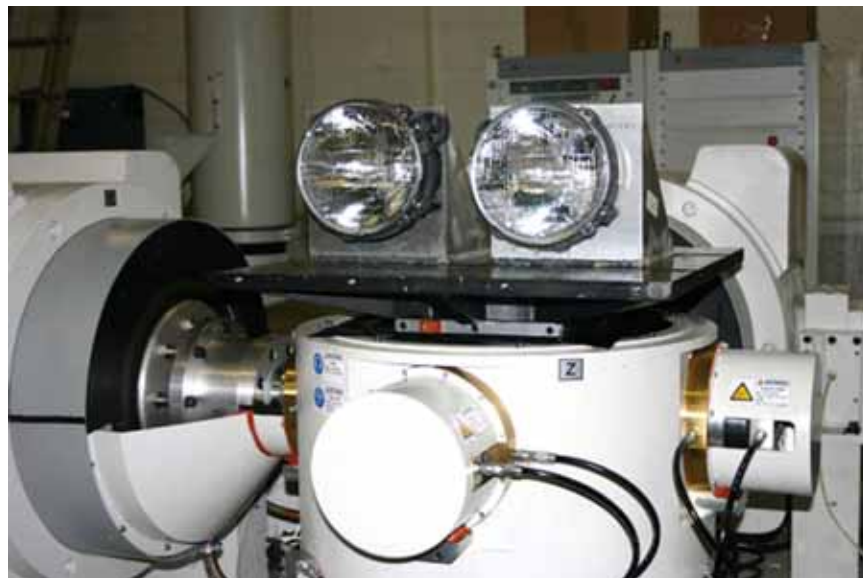
Figure 12 - The motions of three ED shakers are combined into multiaxis shaking.
