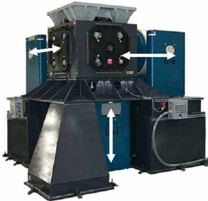
Figure 10 - Three on-site-assembled ED shakers for multiaxis testing of airborne torpedoes. courtesy Naval Underwater Warfare Center, Keyport, WA
