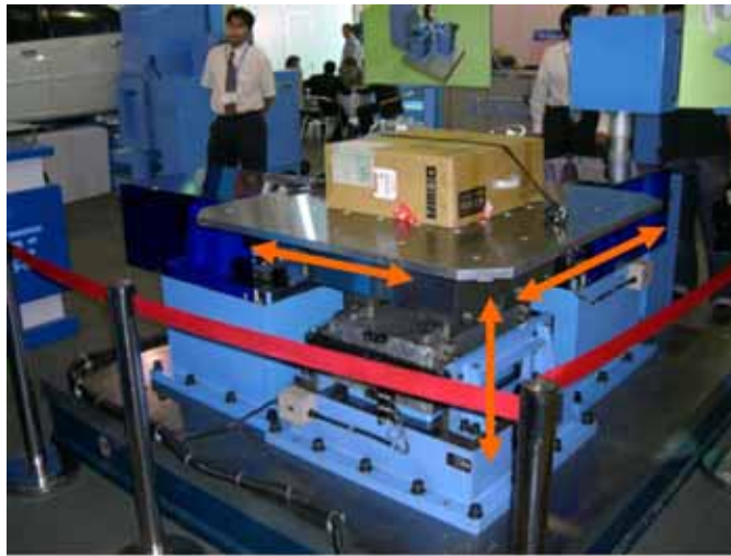
Figure 1 - Sine and random shaking are possible with multiple axis servomotors. The author added three bidirectional arrows. courtesy Kokusai
