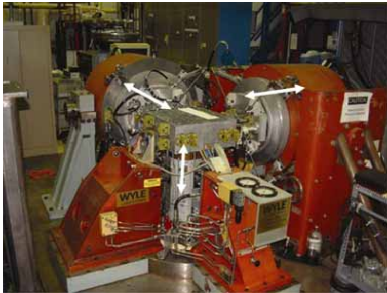
Figure 8 - This pioneer grouping of three ED shakers suggests the complications of on-the-job assembling of three ED shakers, permitting simultaneous multiaxis shaking without damage to any of the shakers.
