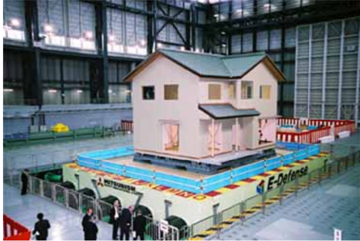
Figure 5 - Seismic investigation of residence (courtesy Mitsubishi Heavy Industries LTD.)
