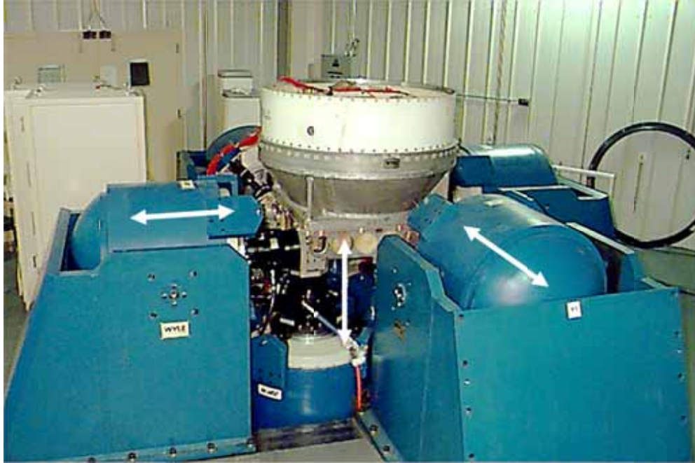
Figure 25 - USAF Multiaxis ED shakers (Courtesy U.S.A.F.)
