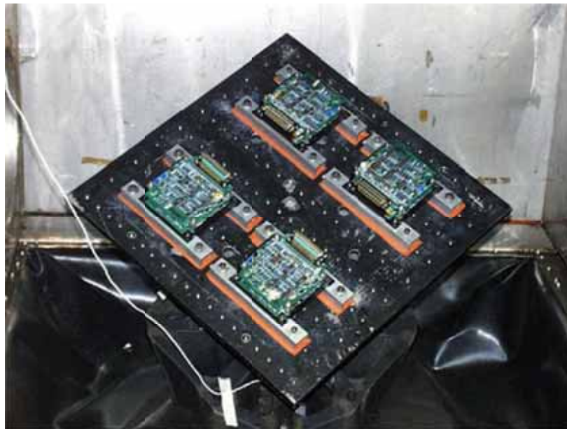
Figure 13 - Some labs tilt their test articles (courtesy Hong Liu)
