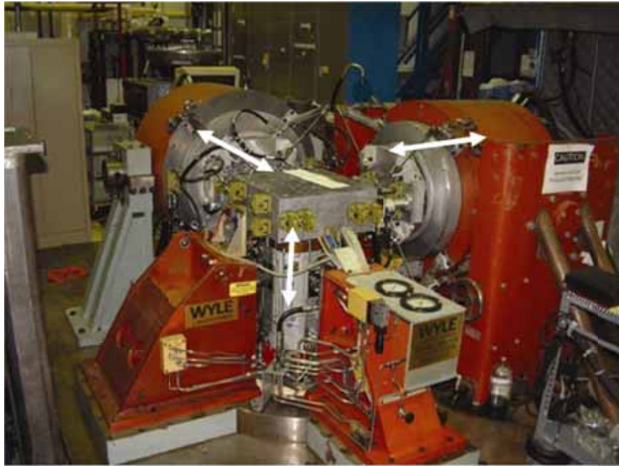
Figure 23 - Pioneer three-shaker 3DoF realization (courtesy US Army)
