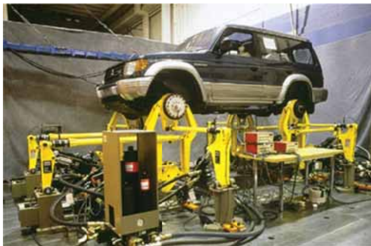
Figure 9 - Road simulation on automobile (courtesy MTS)
