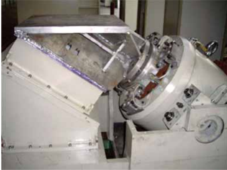
Figure 14 - Tilted single-axis shaker maintains normal gravity loading of the test article (Courtesy Quanta Labs)
