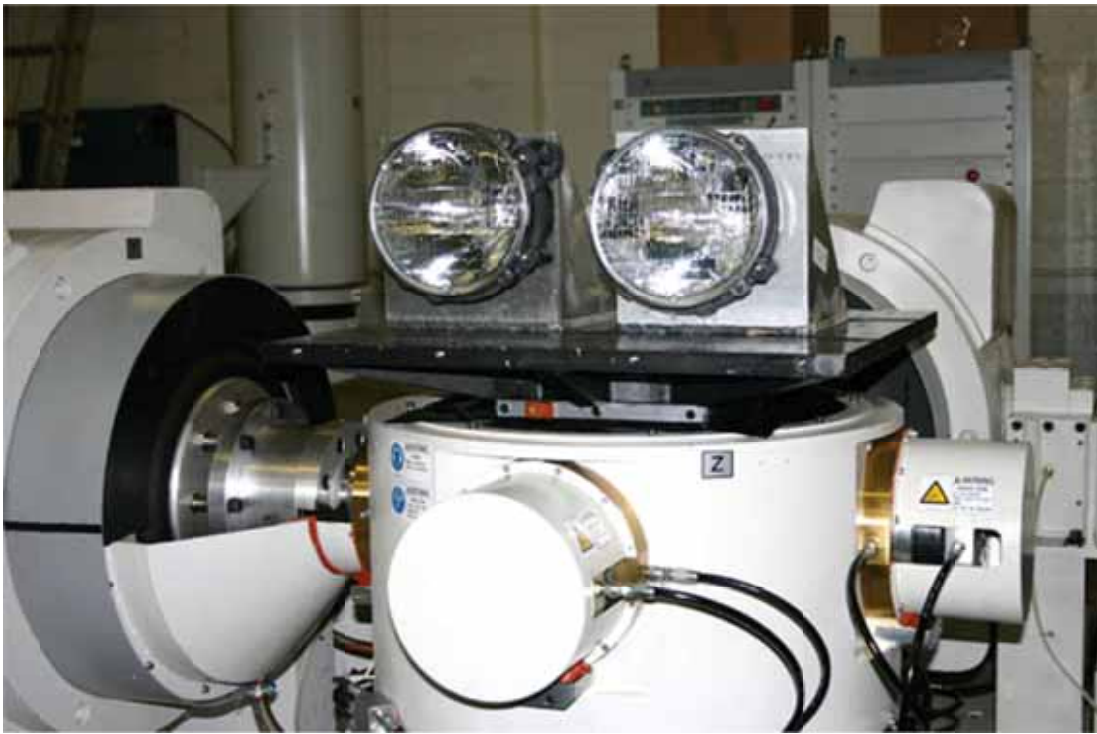
Figure 19 - Triaxial shaking of automobile headlamps (courtesy Spectrum Technologies)
