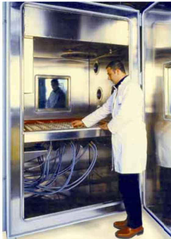
Figure 15 - RS actuators combined with thermal chamber (courtesy QualMark)
