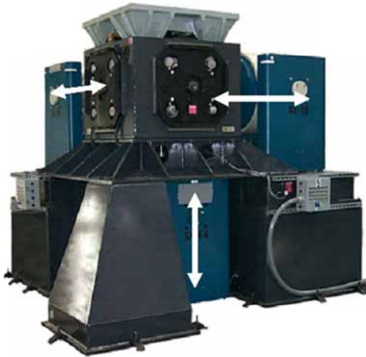
Figure 27 - Three-shaker Navy 3DoF realization (Courtesy NUWC Keyport and Baughn Engineering)
