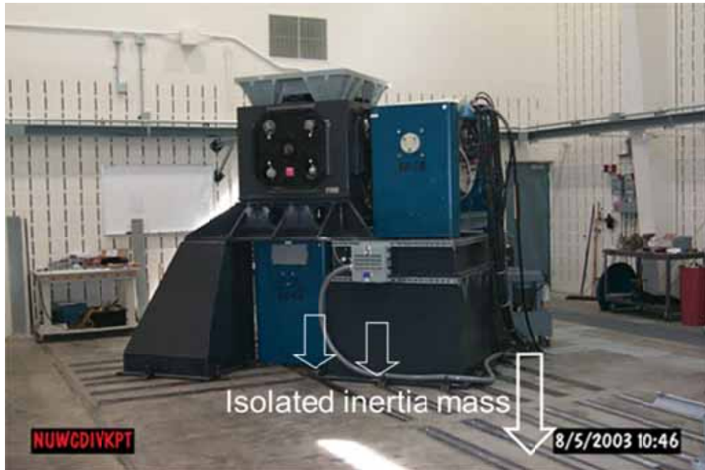
Figure 29 – Three shakers are attached to isolated inertia mass (Courtesy NUWC Keyport and Baughn Engineering)
