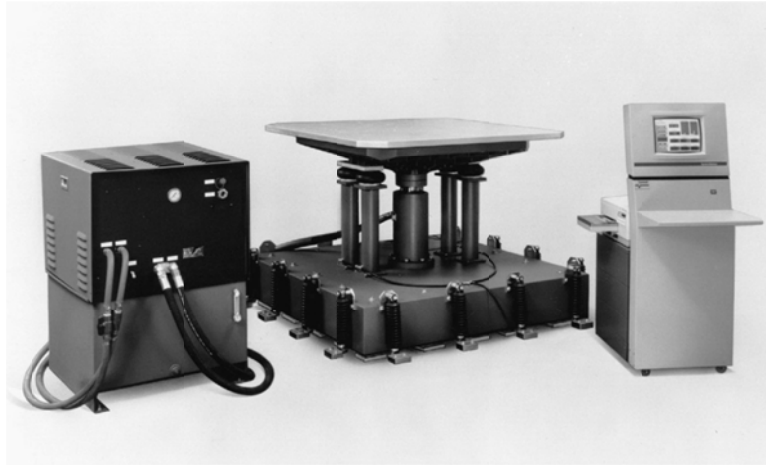
Figure 3 - Servohydraulic vibration system (courtesy Lansmont)
