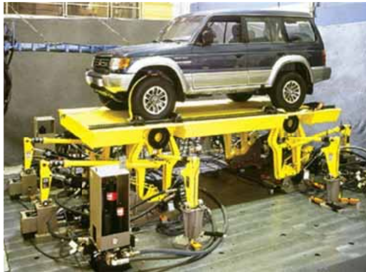
Figure 8 - Platform simulates rail or other transport (courtesy MTS)
