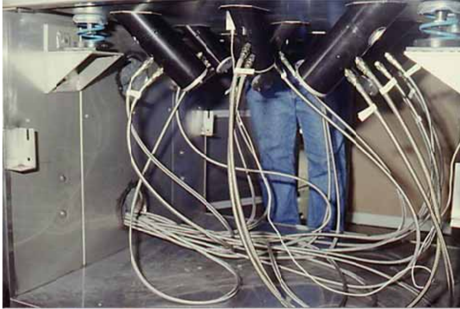
Figure 16 - Pneumatic RS units excite the softly-sprung platform (courtesy GHI)
