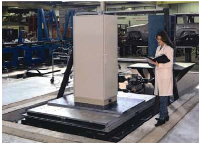
Figure 4 - Horizontal NEBS testing (courtesy Dayton T. Brown)
