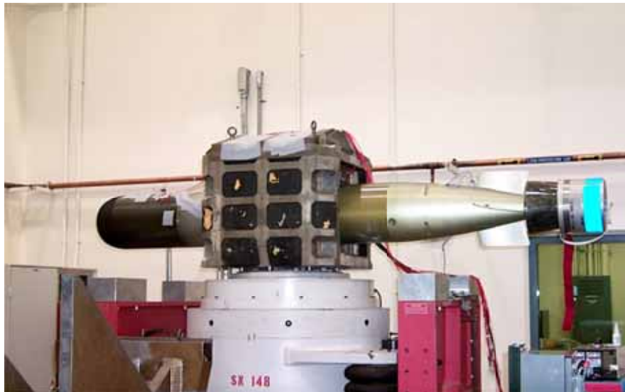
Figure 34 shows earlier single shaker vertical single-axis excitation of fixture and torpedo. The torpedo needed to be supported from above, as when carried by torpedo bomber aircraft. (courtesy NSWC Keyport)
