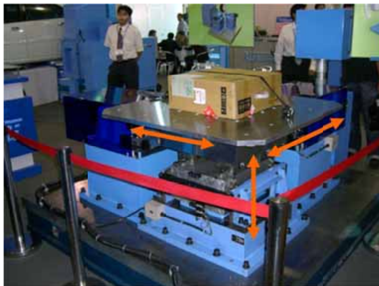
Figure 2 - Three-axis vibrating platform (courtesy Kokusai Keisokuki)
