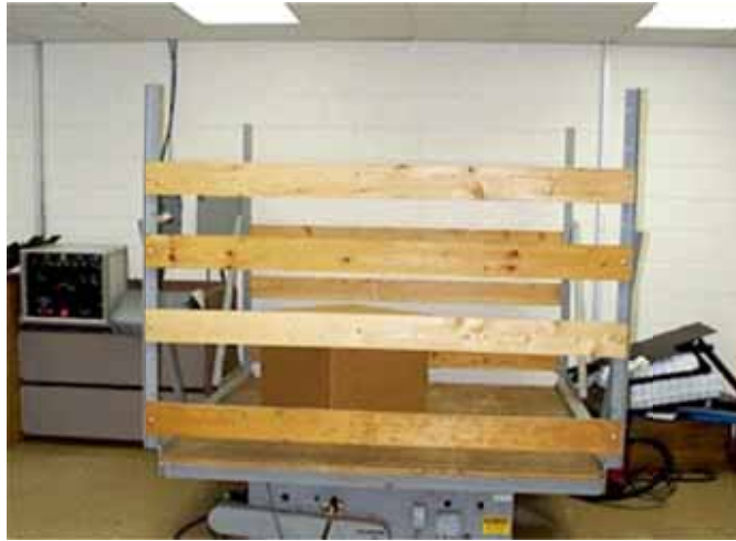
Figure 1 - Mechanical vibrating platform (courtesy LAB)
